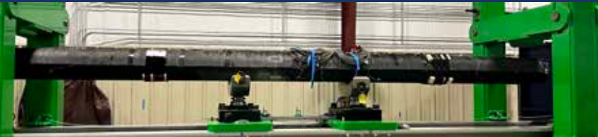
DFOS instrumented gas pipeline testing
