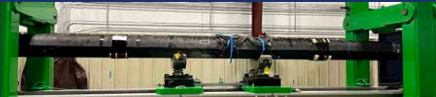
DFOS instrumented gas pipeline testing
